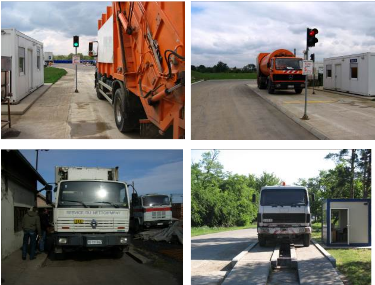
Picture 1.1: Measuring trucks on weighbridge
